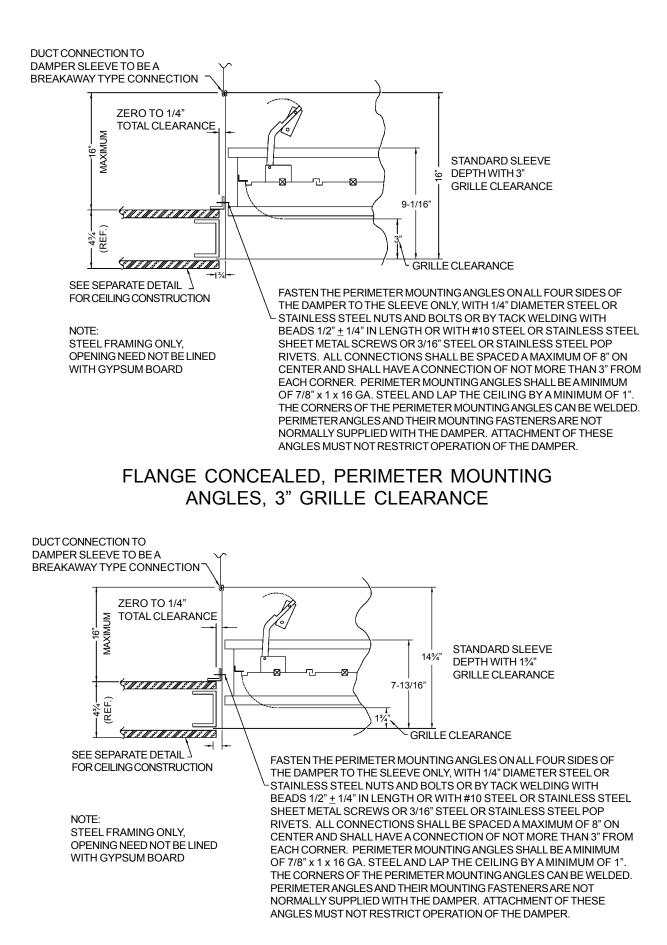
FLANGE CONCEALED, PERIMETER MOUNTING ANGLES, 1¾" GRILLE CLEARANCE
