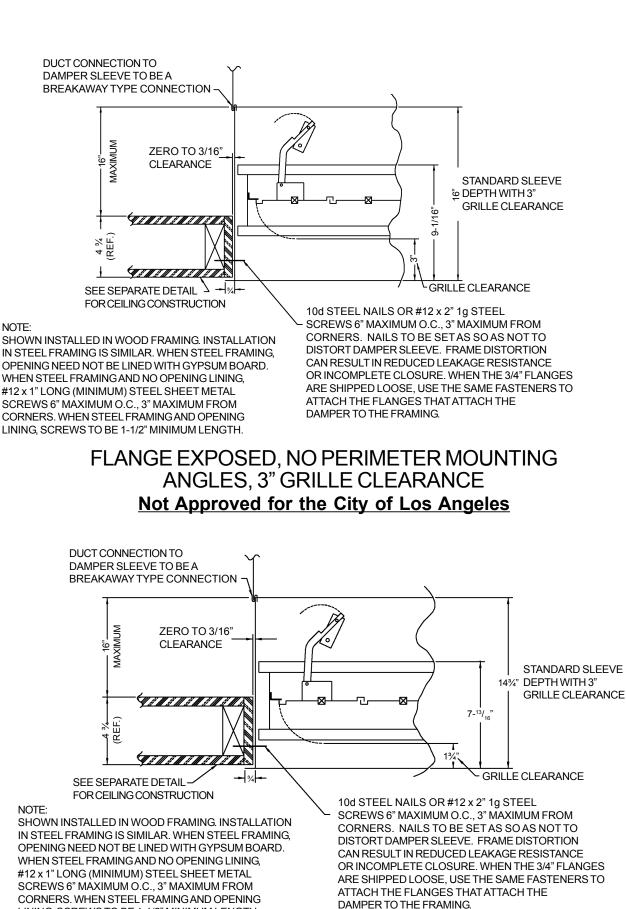
FLANGE EXPOSED, NO PERIMETER MOUNTING ANGLES, 1<sup>3</sup>/<sub>4</sub>" GRILLE CLEARANCE Not Approved for the City of Los Angeles
