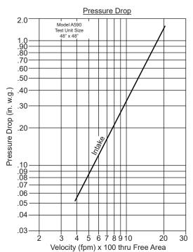
Intake air converted to standard air density. Tested to AMCA Standard 500-L, Figure 5.5.
