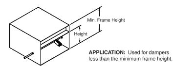
**B-PAN:** 24-GA galvanized steel attached to damper sleeve and caulked at each side.
