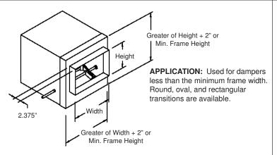
**TRANSITION CAP:** 22-GA galvanized steel attached to damper sleeve and caulked.
