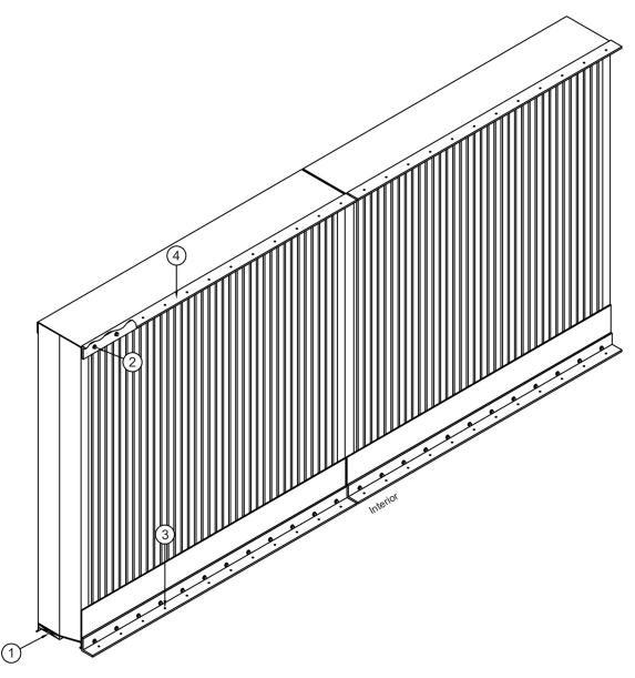
All fasteners must be A307 plated steel or 304 stainless steel.
