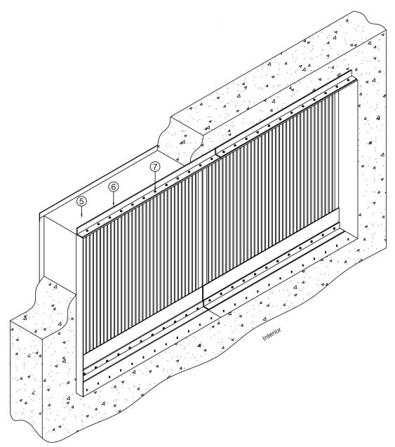
All fasteners must be A307 plated steel or 304 stainless steel.
